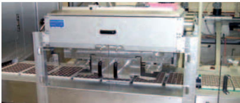
Production example: In the candy machines from Winkler and Dünnebier, RFID guarantees that there is an overview of all forms used at all times
