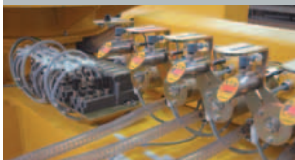
Lubas uses 53 pressure sensors and two BL67 I/O stations in its 15t vacuum traverse Page 34
