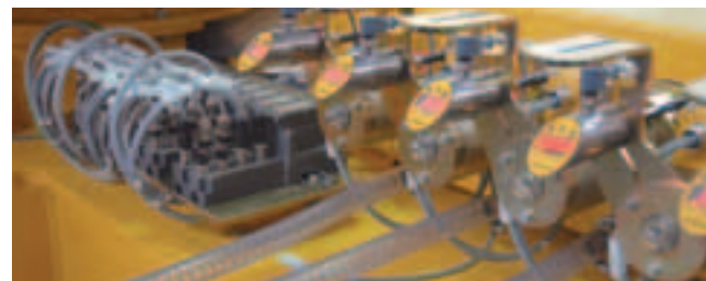
53 pressure sensors and two BL67 I/O fieldbus stations process the signals from each individual vacuum suction cup
