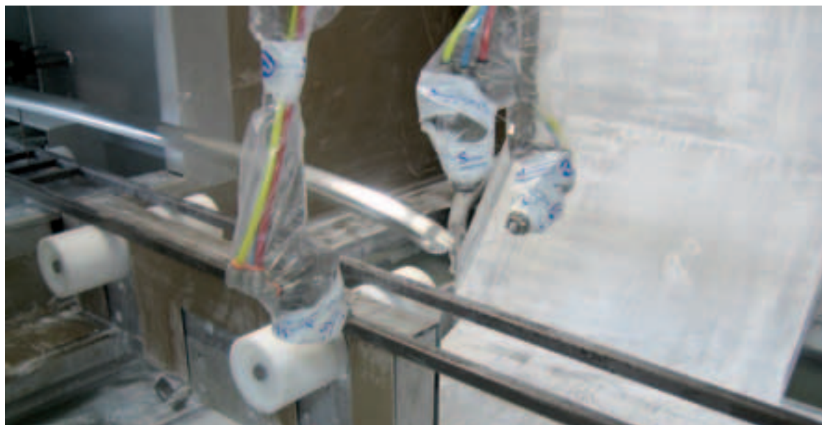
The spray nozzles must approach the molding precisely so that a high quality coat of paint is guaranteed
