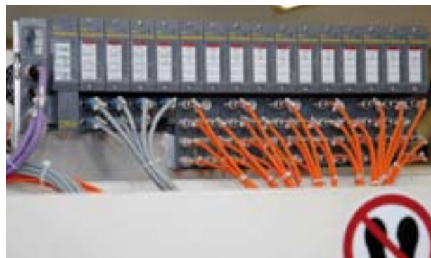
FRIMO uses Turck's I/O system BL67 also for transmitting high frequency signals Page 18
