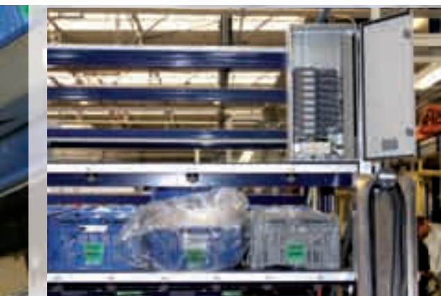
The Pick-to-Light modules from each picking station are controlled by a separate SPS – the Turck I/O System BL67 ensures reliable signal transmission
